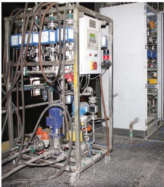
Figure 13: Mobile mixing and metering module
