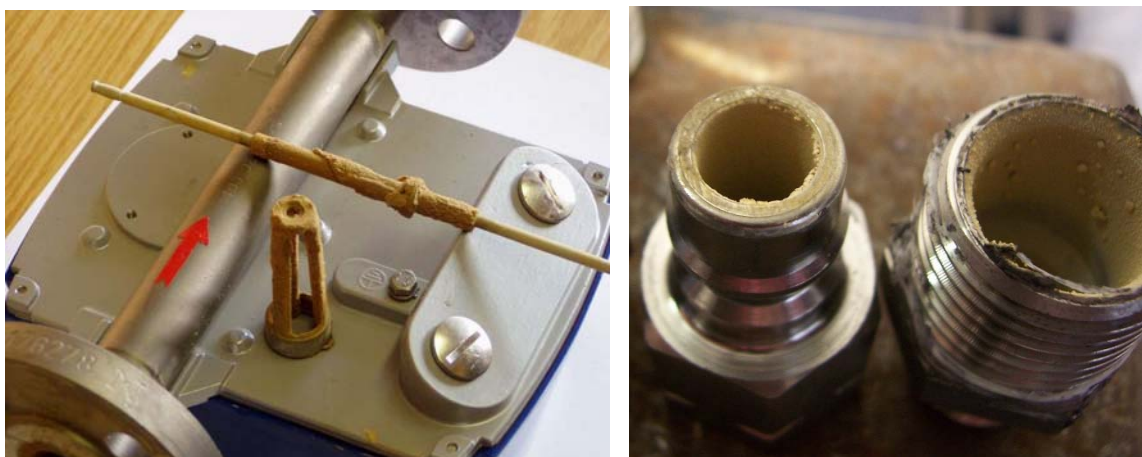
Figure 14: Deposits Caused by Lime Precipitation
