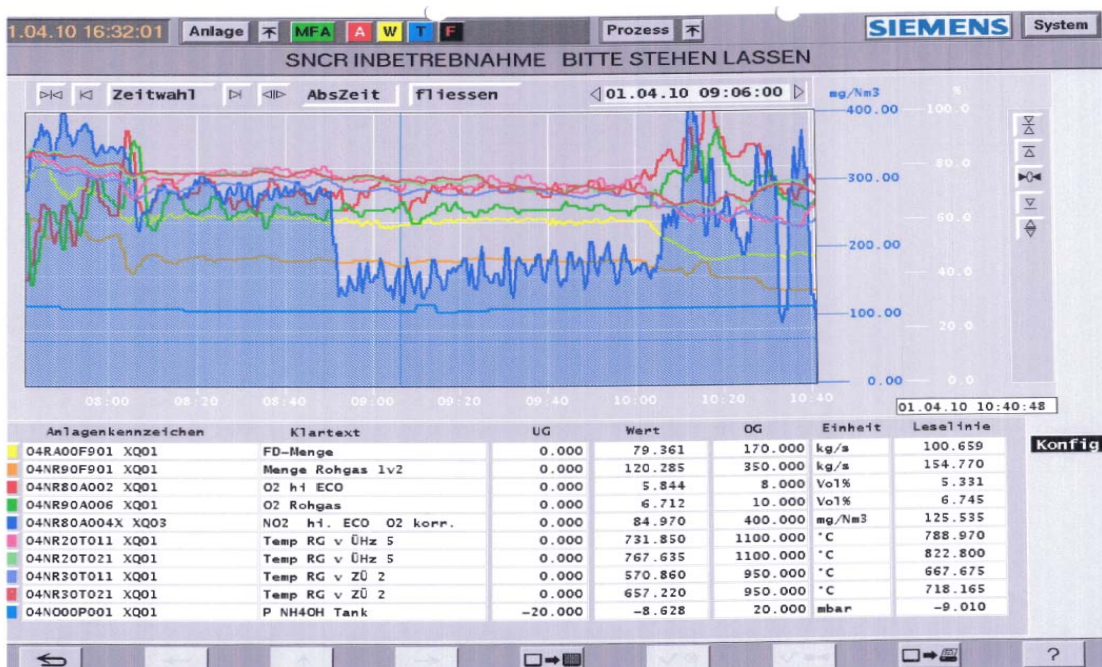
Fig. 9: Operating Results with SNCR Plant in 200 MWel Coal fired Boiler
