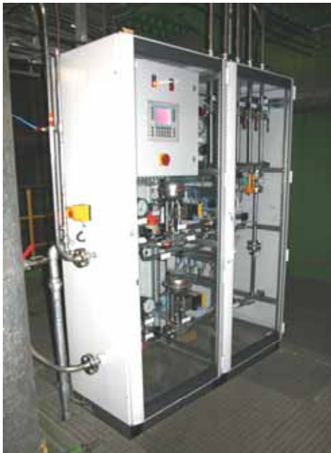
Fig. 16: Metering and Mixing Module
