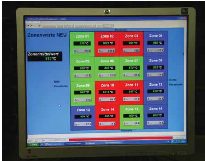
Fig. 11: agam - Configuration of 16 Temperature Zones
